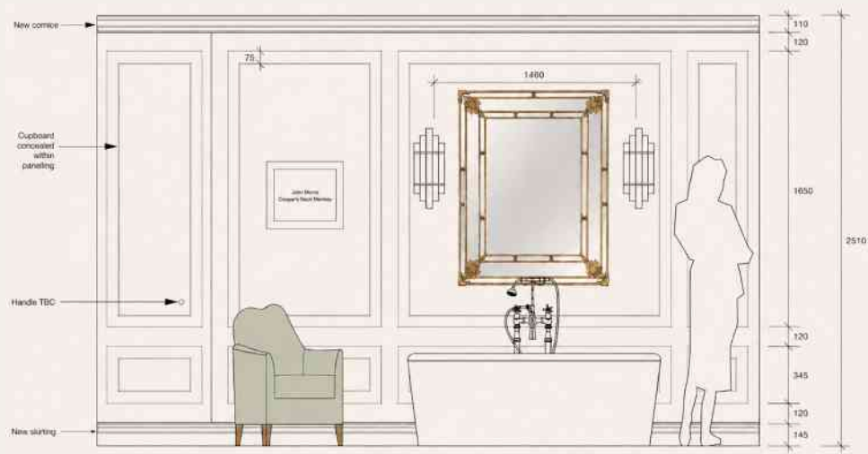
bath wall elevation
